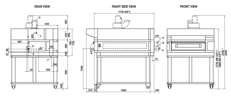
NOTE: The dimensions indicated in the views are in millimeters. \*Dimensions refer to the oversized hood.
