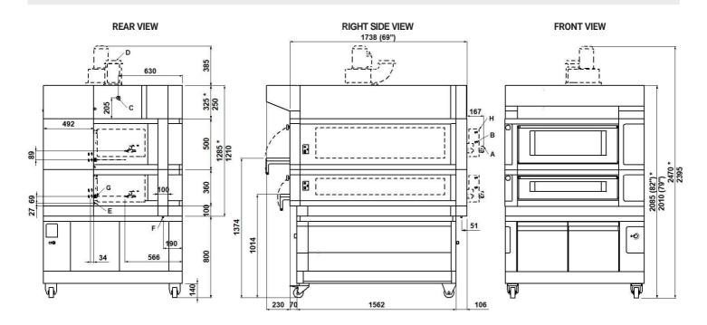
NOTE: The dimensions indicated in the views are in millimeters. \*Dimensions refer to the oversized hood.
