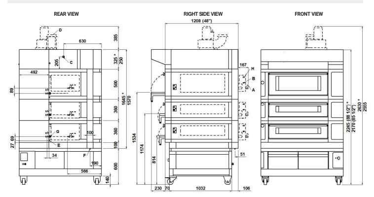
NOTE: The dimensions indicated in the views are in millimeters. \*Dimensions refer to the oversized hood.
