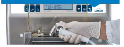
The **delayed cleaning program** guarantees hygienic by controlling the temperature of the cylinder once the gelato has been extracted. So immediate washing of the machine is not necessary in the event of prolonged work stoppages.
