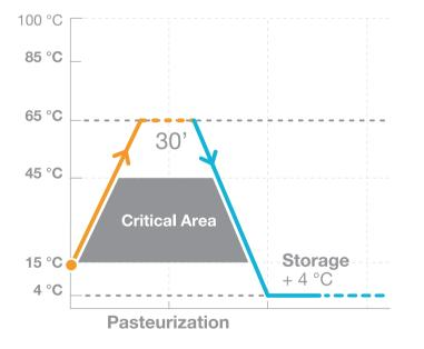
**Standard**. With the automatic **self-pasteurization** system you can choose when to wash the machine up to a maximum interval of 42 days. As a further guarantee of hygienic safety, if the operator does not perform the complete cleaning at the end of the set days, the machine goes into automatic block.
