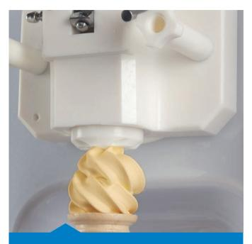
**Star Door** Allows the use of the new nozzles and the single-portion kit. **Monoportion kit** Kit of nozzles suitable for filling small cups, cannoli and other frozen dessert monoportions.
