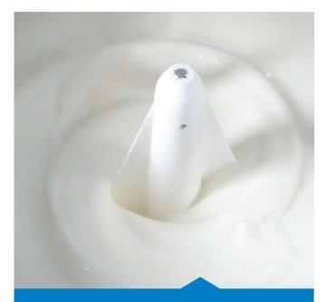
Tank agitator with adjustable speed Prevents stratification during storage and improves heat exchange during pasteurization.
