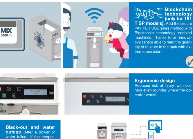
**outage.** After a power or water failure, if the temperature-time parameters guarantee that the mixture has not undergone any alteration, the machine resumes the program in progress. Otherwise, if the machine is self-pasteurizing, a pasteurization cycle is automatically started, warning the operator with a message on the display. In the case of the non self-pasteurizing version, the machine requires washing.
